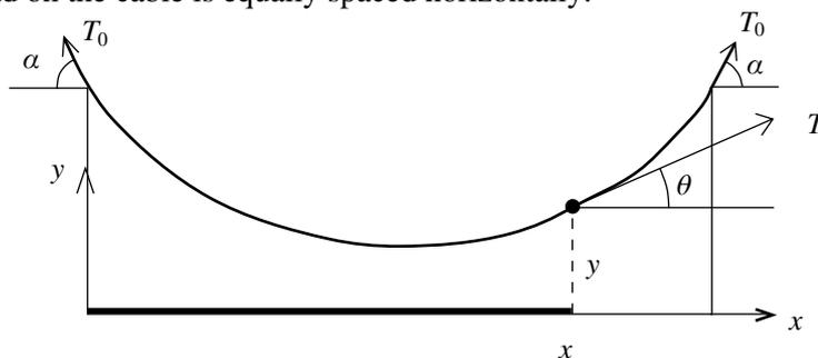
2. Show that the load borne by the cables up to a point distance  $x$  from the beginning of a bridge of length  $l$  is  $Wx/l$ .
